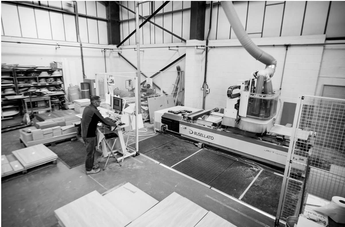
Fig. 24_ Off site fabrication, CNC of panels at i4Detail Ltd
