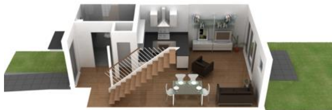
Fig 13 The BoKlok house type shown above is the Alsten, this is the mid sized dwelling with a 2b3p (two bed three person) format. The bedrooms are larger in this particular house type. The ground floor living and dining spaces are also larger and allow for greater storage options and flexibility of space.
