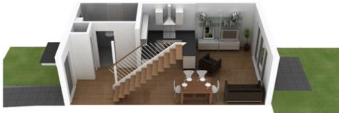
Fig 12a. The BoKlok house type shown above is the Molna, this is the 'base unit' for the larger dwellings within the BoKlok house type range. The planning and location of primary walls are shared with the larger house types. The minimal changes to this base format affords the option of larger dwellings with minimal constructional and manufacturing stages, reducing costs and time to build different house types for a proposed site.
