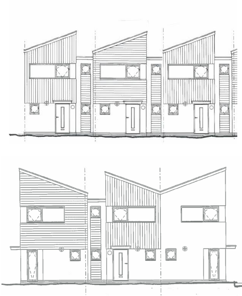
Image.21. The elevational treatment for each dwelling has been formatted to allow for different 'zones' of the facades to be inter-changeable in terms of materials used in differing locations. For example in the UK, the Boklok house types are mainly constructed using a render and timber paneled appearance. This is very acceptable to many of the Boklok sites in the UK in terms of planning conditions. However, across Europe these areas of the façade can be clad in a 'Trespa' panel system (coloured Aluminium composite panel). To add variety but reducing the number of external materials, the location and direction of the cladding is amended. The example above with a streetscape of three Alsten dwellings has variety of external appearance by mixing vertical and horizontal timber cladding.
