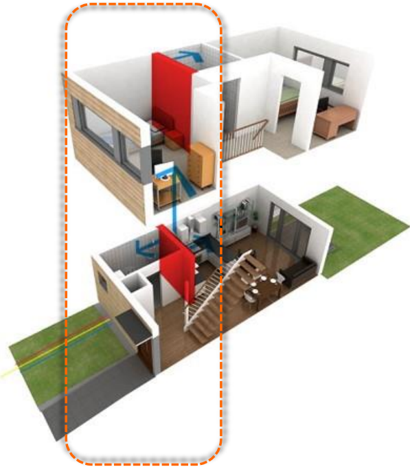
Fig 17. The BoKlok house type has been designed with many elements of the design allowing for repetition of service locations and routes. All socket locations have been fixed at agreed locations. These locations can be altered when the open panel system is used. The open panel system leaves the internal element (plasterboard) to be completed on site, allowing for maximized option for change.
