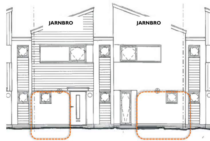
Image.22. The elevations above show the removable external panels that allow for future podularisation of internal rooms. For example the rooms that often require refurbishment are the bathrooms and kitchens as these get high use. By removing the external panel(s) the room 'pod' can be quickly removed and a new pod fitted. The external rendered panel is then replaced.
