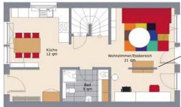
Fig 4. The BoKlok house type at ground floor has a plan form that minimizes the circulation floor area allowing for greater usable floor area for 'living' spaces. The relationship of living space to circulation space is improved by 22% over similar house types of comparable floor area. The wet spaces are retained in one define 'room'. This room affords the dwelling a ground floor wc and shower room, combined with a utility area.
