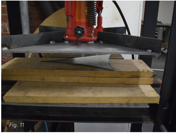
Fig. 11 (above) the flat form of the 1:8 scale mild steel maquette in the rig prior to hydroforming.
