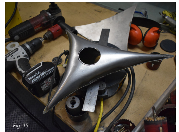
Figs. 13-15 (below, l-r) the oculus is cut out of the hydroformed 1:8 scale mild steel maquette. (SM)
